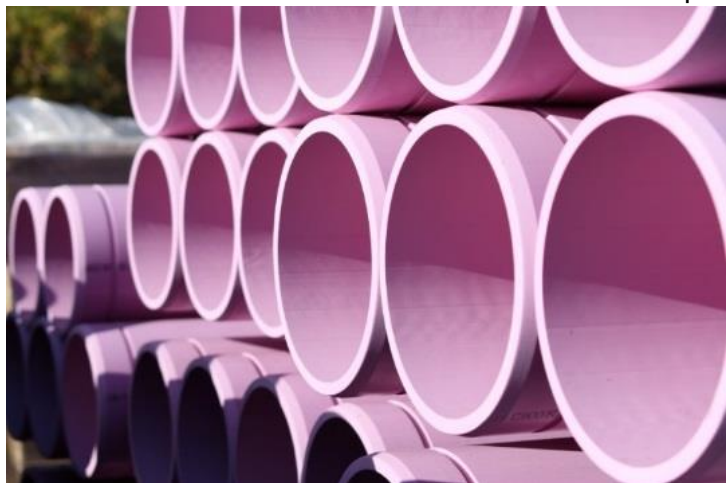
Reclaimed water pipes
