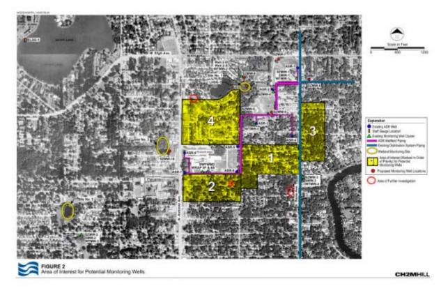
FIGURE 1 Locations of ASR Wells and Existing and Proposed Monitor Wells at the Tampa-Rome Avenue Park ASR System. Figure from CH2M HILL (2006)
