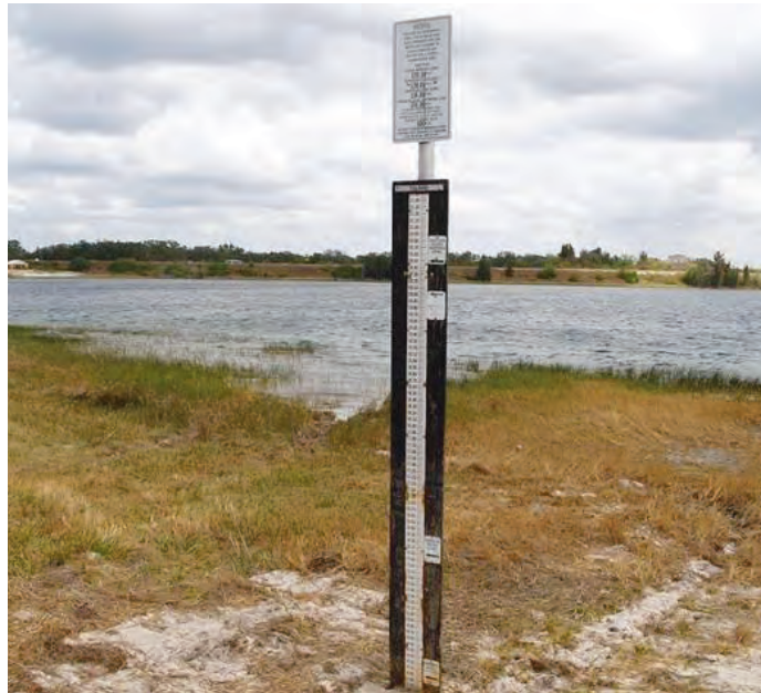
A staff gage on a lake in the Lake Wales Ridge illustrates the problem of low lake levels that have resulted from successive droughts and groundwater pumping.
