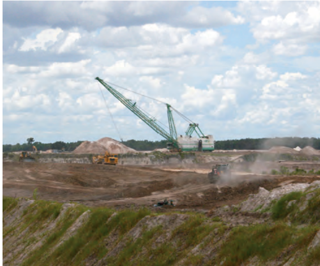
A dragline mining phosphate ore in Hardee County. Demand for water for mining and other Industrial uses is projected to increase by more than 6 mgd during the planning period in the Heartland Planning Region.
