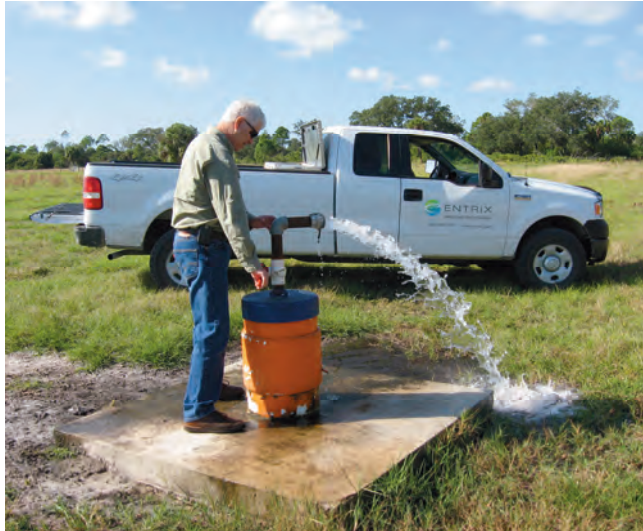
A technician checks the flow and quality of groundwater from a naturally flowing well in southern Sarasota County.
