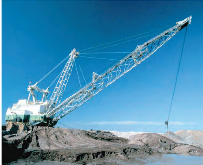
A dragline mining phosphate ore in the southern portion of the District.
