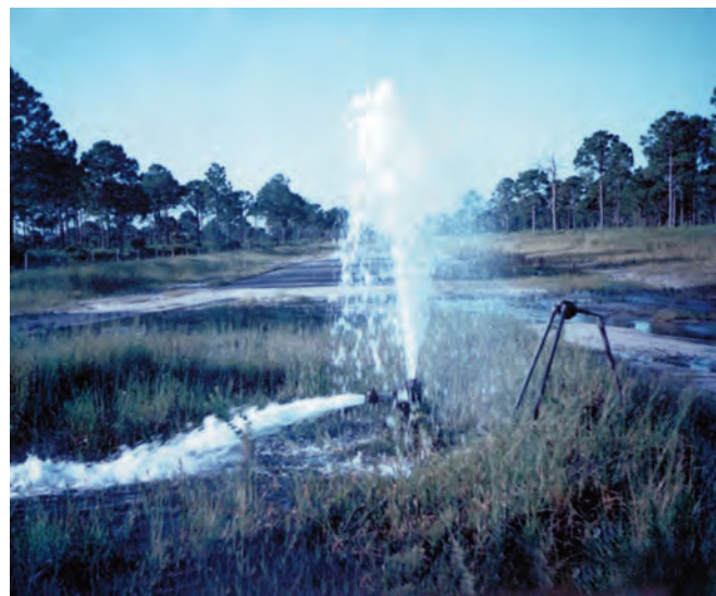
Artesian conditions in the Upper Floridan and intermediate aquifers in the southern portion of the District can cause wells to flow at high rates.
