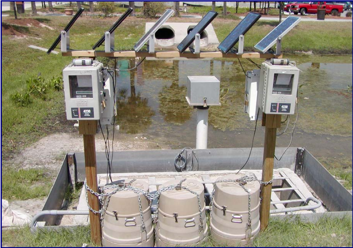
Picture 7 – West view of pond from outflow. In foreground are the flowmeters and samplers for the outflow weir and underdrains. In the background is the shaft encoder, then the equalizer pipe leading to the other half of the pond and inflow.
