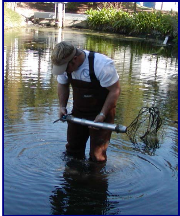
Picture 9 – Preparing to take a sediment sample with corer.
