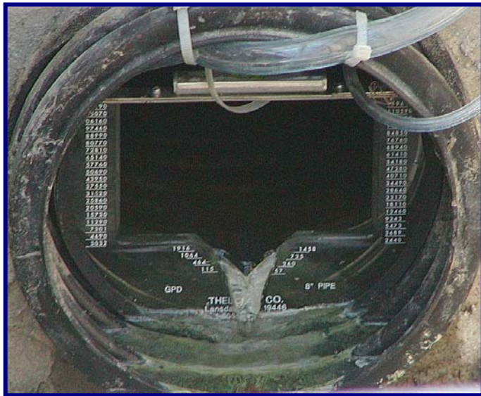
Picture 5 – Underdrain weir with sampling and bubbler tubing. Picture taken during low flow.
