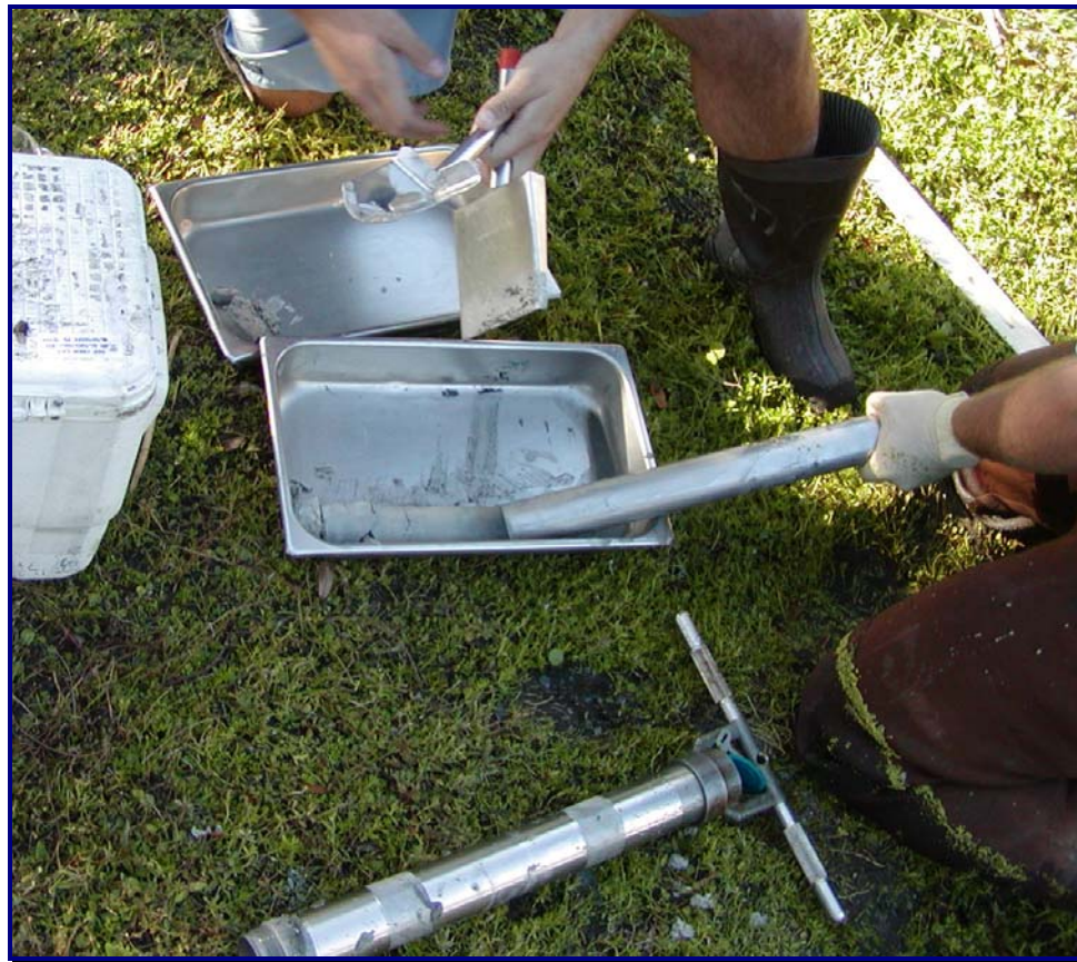
Picture 10 – Resultant core from sediment sampling.
