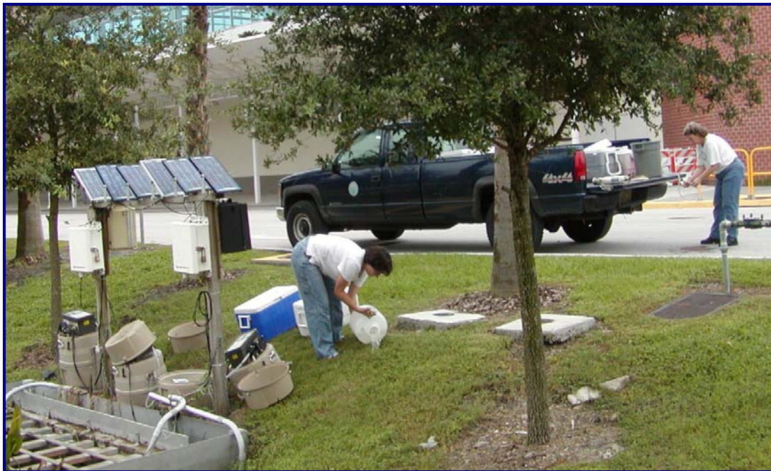
Picture 8 – Routine sampling of the outflow weir and underdrains after an event. The new cruise ship terminal is pictured in background.
